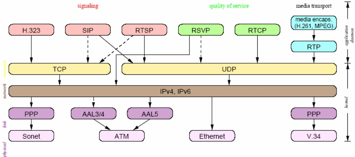
**Fig. 1 Internet telephony protocol stack (Adapted from [2])**
