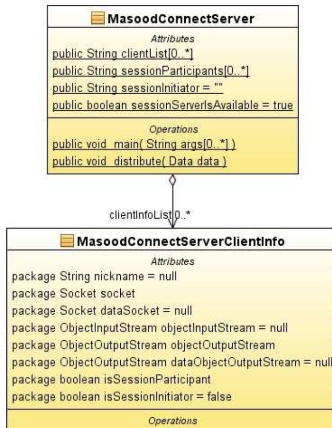
Figure 4: UML Class Diagram [Server-side: Main App]
