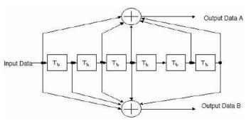
Figure 2. The Convolutional Encoder Used in IEEE 802.11a. From [15]
