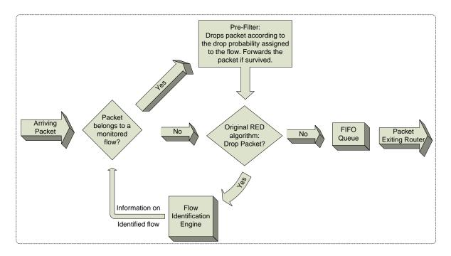
Figure 1: Architecture of a RED-PD router
